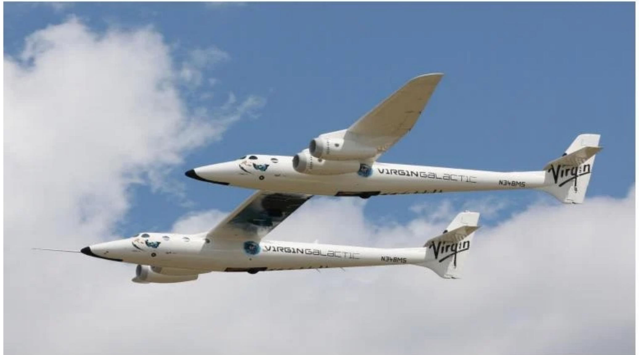
Figure 9: WhiteKnightTwo is a twin mast aircraft used by Virgin Galactic to carry SpaceShipTwo through the atmosphere. SpaceShipTwo is positioned on top of the middle wing, and the combined structure flies from horizontal takeoff to space.
