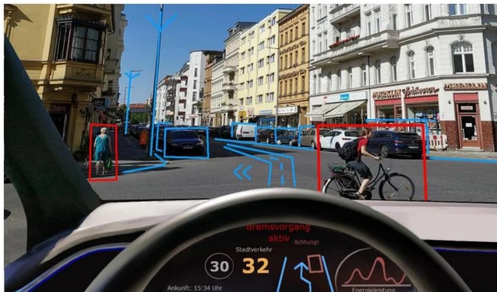
Figure 8: An autonomous car's "mind": it uses machine learning to detect different objects, lane markings on the road, pedestrians, and more.
